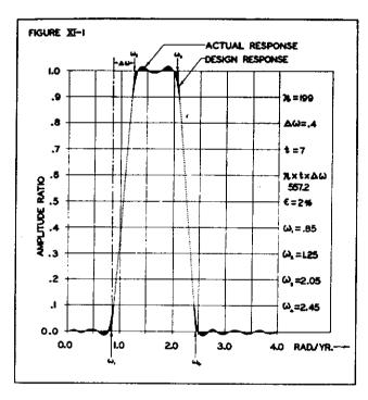
A Typical, Digital-Filter Response Curve
